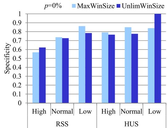
Figure 6. Specificity of MaxWinSize-approach vs. UnlimWinSize-approach (no aging, i.e. leak rate  $p = 0\%$ )
