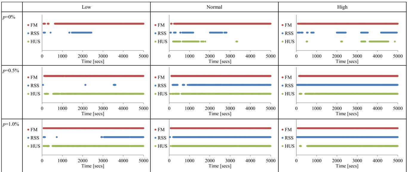
Figure 4. Time charts plotting the aging detection time point for UnlimWinSize-approach; a plotted dot shows that the Mann-Kendall test has confirmed trend at this time point (plotted separately for FM, RSS, and HUS)
