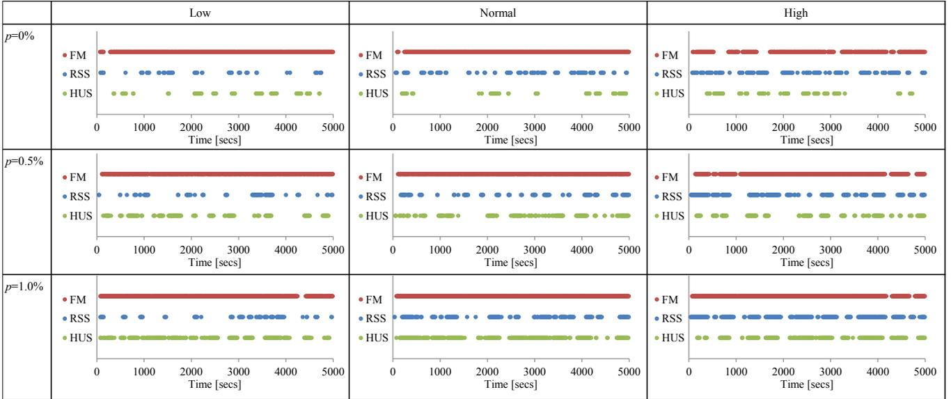
Figure 3. Time charts plotting the aging detection time points for MaxWinSize-approach; a plotted dot shows that the Mann-Kendall test has confirmed trend at this time point (plotted separately for FM, RSS, and HUS)
